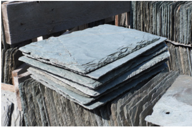
▲ Roof repairs incorporated salvaged slate tiles, those naturally weather-worn, to best match existing ones.
